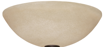
LK80LEDXXX AMBER MIST (4.25" H X 12.38" W) One 16 Watt L.E.D. array Light Output: 1,200 Lumens Color Temperature: 2,700 K Color Rendering Index: > 80
